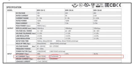
Check AC input current spec of **SDR-120-24** and do calculation with the rated current of ICL-16 16A/0.7A = 22.8... 22 units
