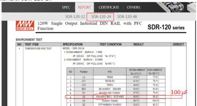
Check C5 capacitor value and do calculation with acceptable capacitive load of ICL-16R  $_2500\,\mu\text{F}/100\,\mu\text{F}=25$   $\Longrightarrow$  25 units
